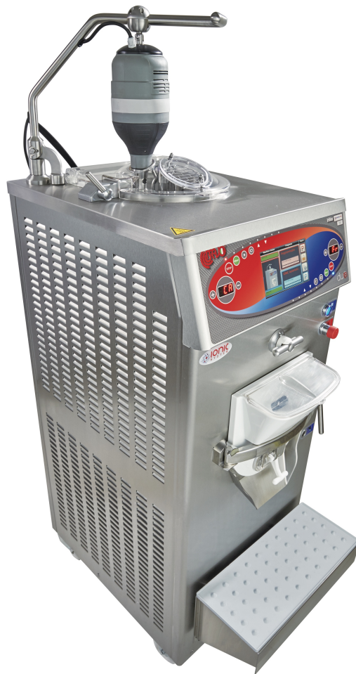
Pic. 13 Combined machine capable of mixing, pasteurizing, homogenizing, cooling down and batch freezing. Photo courtesy of © BRAVO spa.
