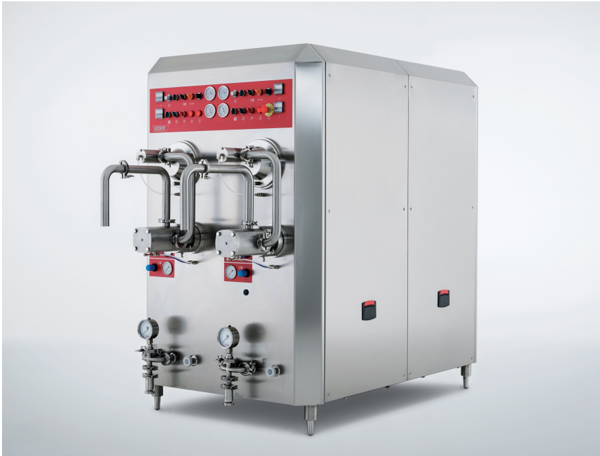
Pic. 8 Continuous freezer model RFE400A / 2 (twin barrel). Photo courtesy of © ROKK processing ltd.
