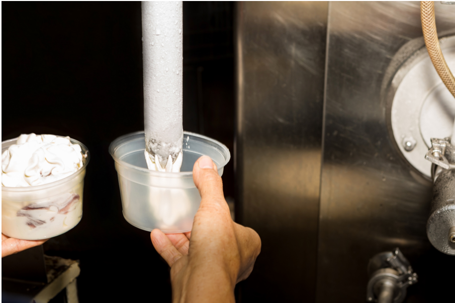
Pic. 16 Detail of a small tubs filling apparatus. The pipe is fed by a continuous freezer.
