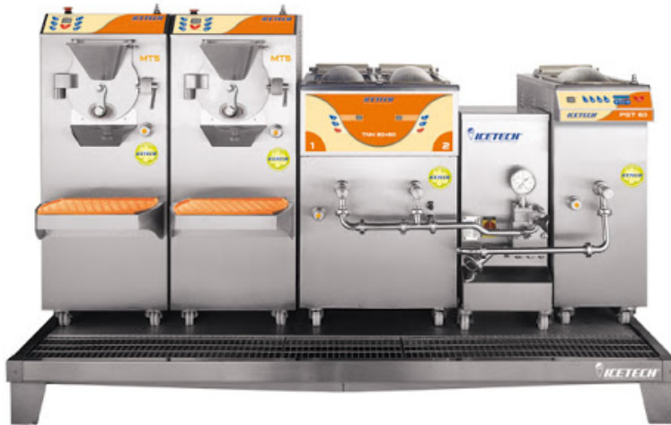
Pic. 4 Full ice cream production line including (from the right): Pasteurizer, Homogenizer, Holding and Ageing device, two batch freezers. Thank to---
