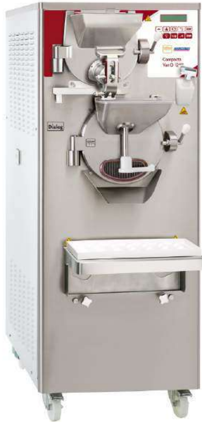
Pic. 75 Combined machine model Compacta VariO 12 Elite. We can see the above cylinder used for pasteurisation, the pouring mechanism and the lower part for the batch freezing. Photo courtesy © Ice Team 1927.
