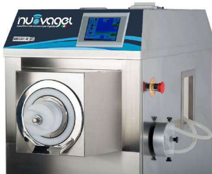
Pic. 76 The new system that uses an Archimedean screw to freeze the ice cream mix. Model "Mantecatore a Vite". Photo courtesy of © LA NUOVAGEL SRL
