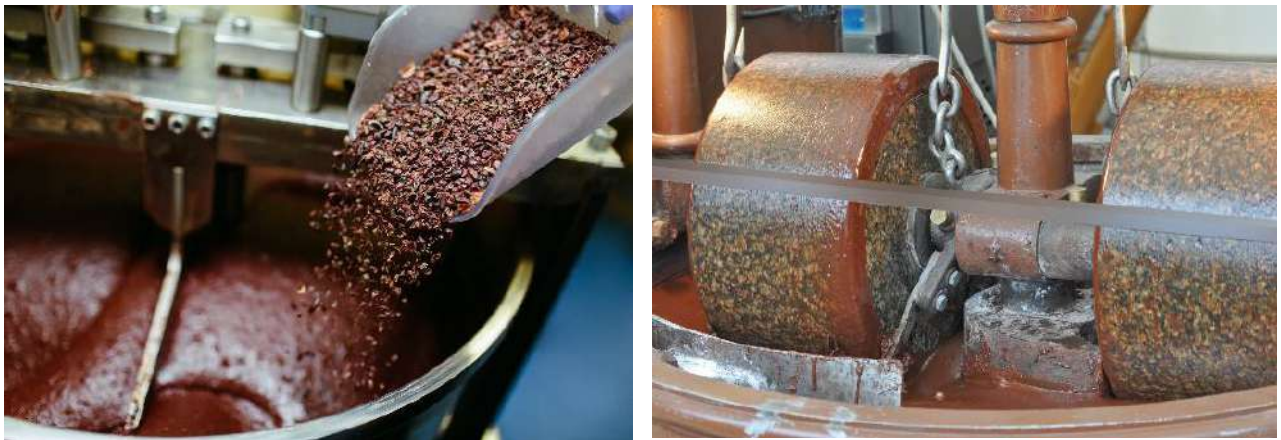
Pic. 50 First grinding and pasting of the cocoa nibs with sugar and other ingredients
